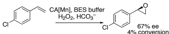
**Scheme 2.** Epoxidation of *p*-chlorostyrene catalyzed by CA[Mn]. Reaction conditions: 30 °C, 16 h, BES buffer (0.1 M), pH 7.2, CA[Mn] (41 mM), sodium bicarbonate (147 mM), *p*-chlorostyrene (7.4 mM), H<sub>2</sub>O<sub>2</sub> (7.4 mM).
