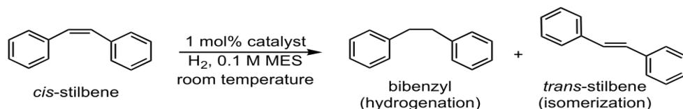
**Scheme 1.** Hydrogenation of *cis*-stilbene with up to 20/1, ratio of hydrogenation/isomerization.
